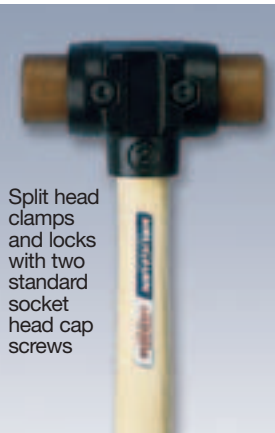
Faces can be rotated for uniform wear and increased life
