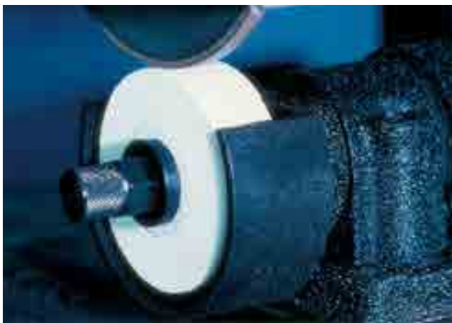
AFTER TRUING THE WHEEL FACE IS SMOOTH AND CLOSED
